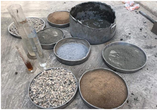
Fig. 1. Raw Materials Used for Concrete Mix.
