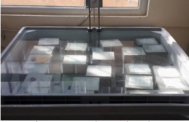
Fig. 3. Concrete Specimens During Curing.
